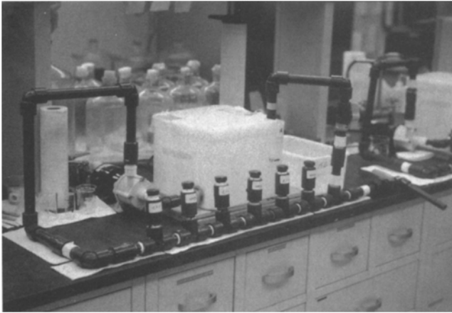
Fig. 1. MAT unit as described in Materials and Methods. High-density polyethylene tank (9.0 l working volume) can be seen with attendant pumping system. PVC bypass loop with coupon holders in foreground.
