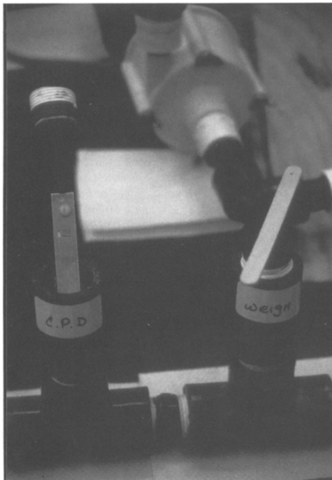
Fig. 2. Close-up photograph of two coupon holders from MAT unit bypass loop. Coupons of 316 stainless steel, brass, or wood were bolted to coupon holders with polyethylene fasteners and lowered into recirculating culture medium.
